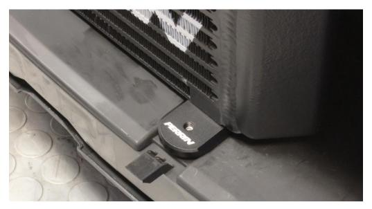
10. Install M6 fender washer then M8 fender washer onto supplied M6 bolts. Pull down lower splash guard and install them up through the holes in the splash guard and into the PERRIN Oil Cooler Brackets. Tighten bolts to roughly 10-15ft-lbs of torque.
