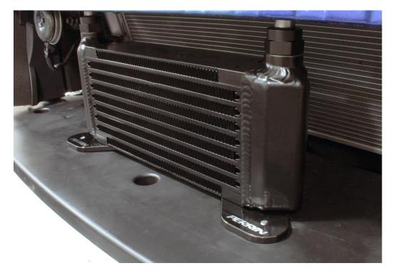
16. Install supplied fender washer onto M6x50 bolt. Install bolt with washers from bottom of car up through splashguard into PERRIN Oil Cooler Brackets. Tighten bolts down to roughly 15 to 20ft-lbs or just beyond hand tight. **NOTE: Do not over tighten these bolts, as they will eventually break through plastic part of splashguard.**
