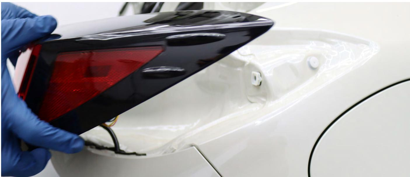
Remove the tail light by disconnecting the plug socket.
