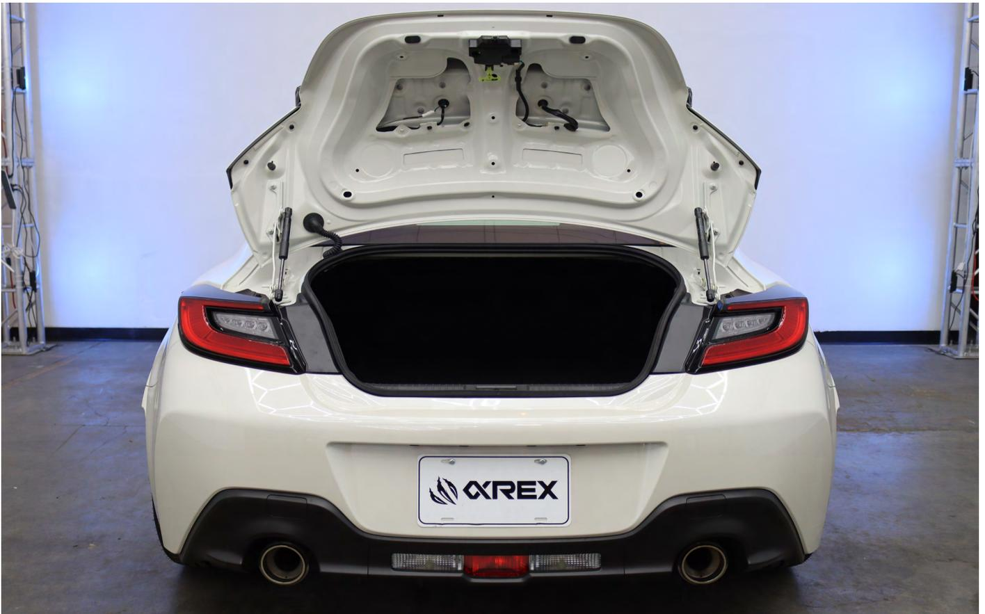
To detach the tail light, begin by raising the plastic guard cover. Loosen the 3 X 10mm bolts by turning them counterclockwise.
