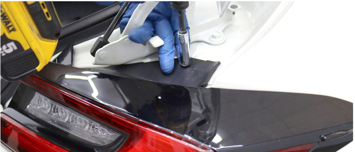
Carefully pull the tail light assembly outward towards you to remove it from its position.
